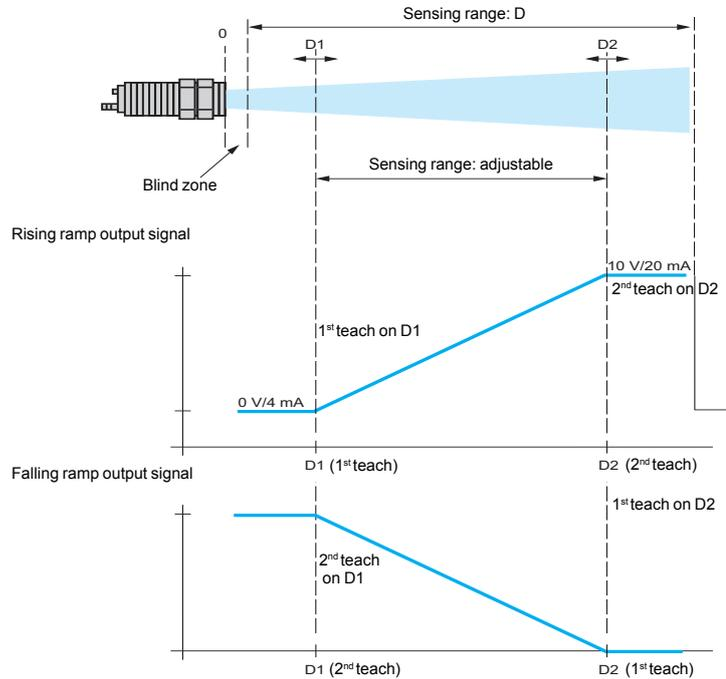
The direction of the slope of the signal is obtained by teaching the first limit:
