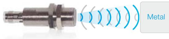
The OsiSense XXV ultrasonic sensor is “Plug and Play”, no adjustment required, no teaching. Its solid-state output changes state when the object to be detected is less than 50 mm away.
